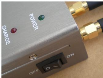
**Red light: when charging for jammer, the indicator light will be on.**
