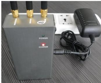
**When the built-in battery is charged full (usually needs 8 hours), the indicator light will be off.**
